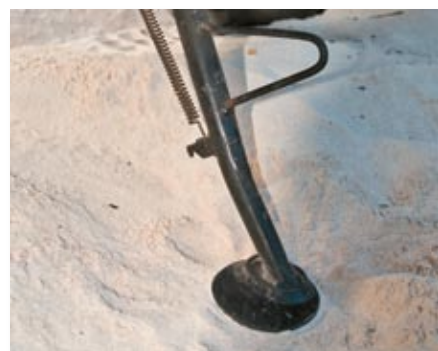
F650GS: Large foot pad on kickstand.
