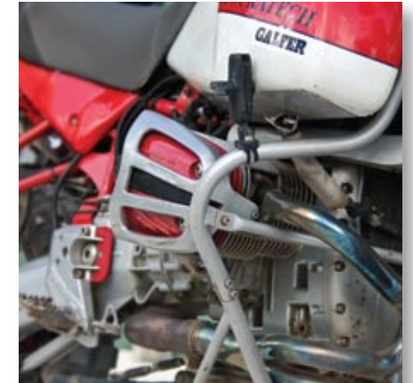
🔧 R1100GS: Engine crash guards and cylinder protectors.
