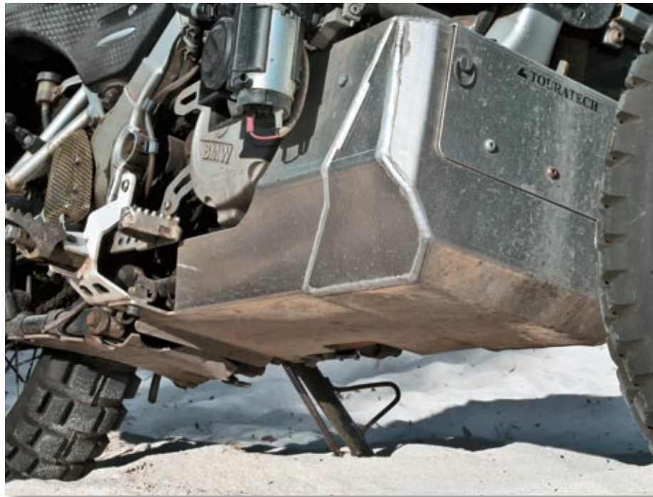
🔧 F650GS: Touratech rally engine sump protector with new, higher sub-frame.
